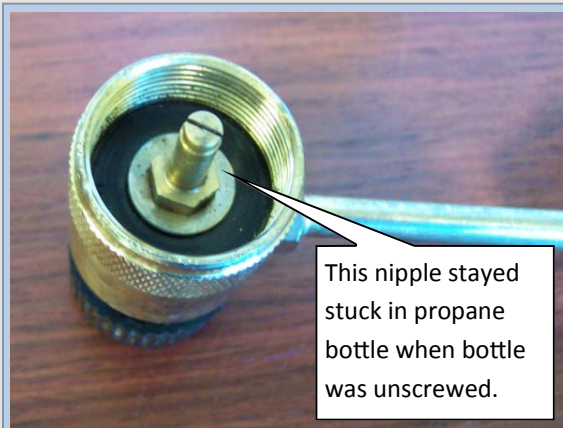
Stove fitting showing nipple piece that became unscrewed from fitting and stayed with mating propane bottle when bottle unscrewed from stove.
