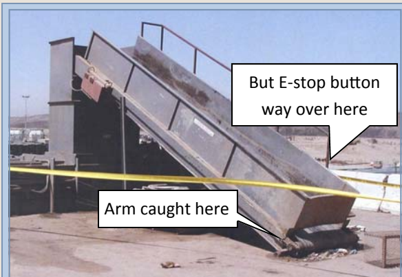
Plastic baler, showing location of injury and relative location of E-stop.
