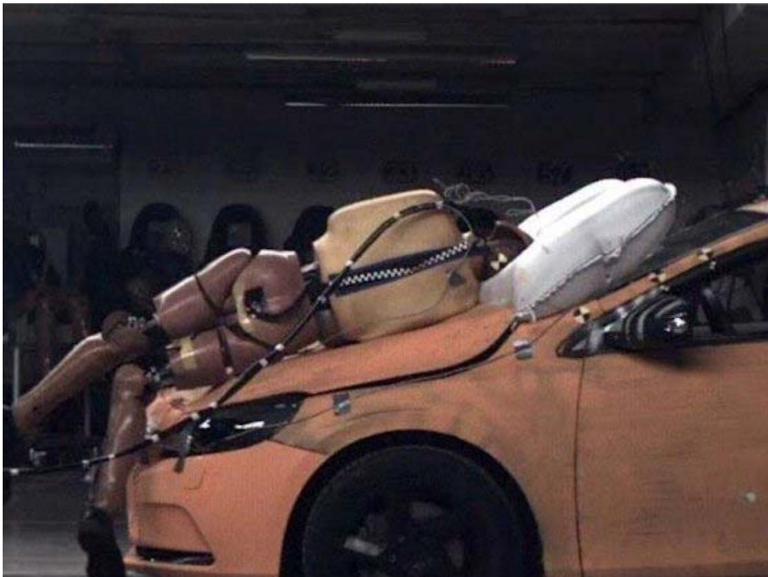
**Protection for the head:** *In Volvo's crash-test center in Gothenburg the results of a auto/ped crash is clear. The head of the pedestrian is protected with an external airbag that is fired by sensors on the front of the vehicle. Severe injuries then are limited to the legs. (Photo: Volvo)*
