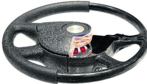
**Safely packed: In an emergency the airbag in the steering wheel should deploy dependably and explode to its full size.**
